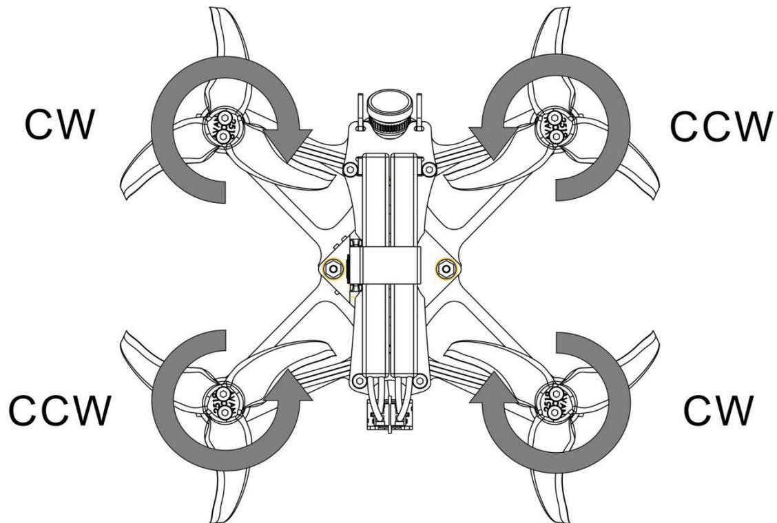
**Caution:** Failure to mount the propellers in the correct orientation will cause Tinyhawk II Freestyle to not fly correctly and with no control. Please double check for the correct orientation.
