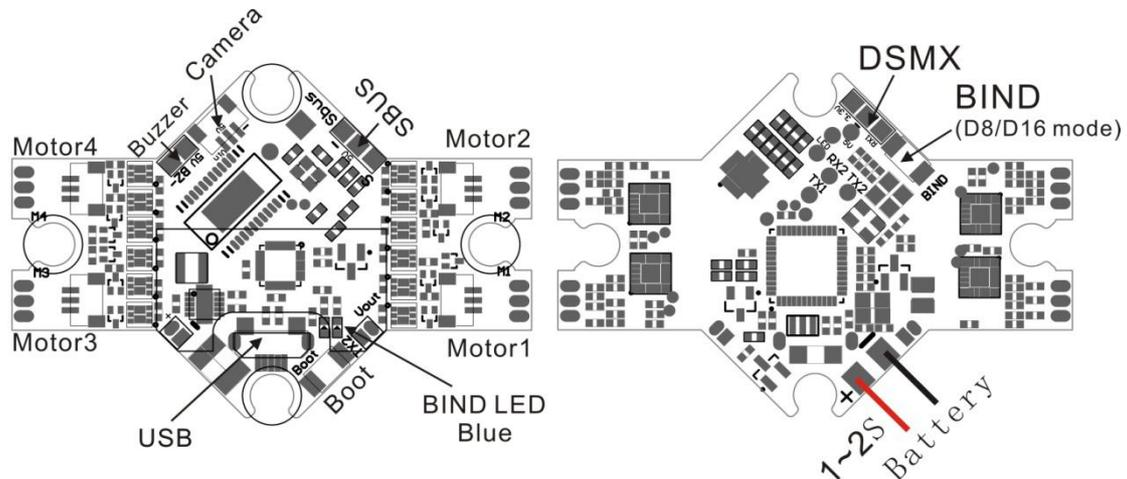
Tinyhawk II Freestyle's main electronic board is shown above. This board contains a F4 flight controller with all 4 esc's and an 8CH receiver.
