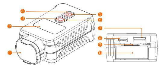
Usens protection hood S Wi-Fi/Menu button **OLED** Display
