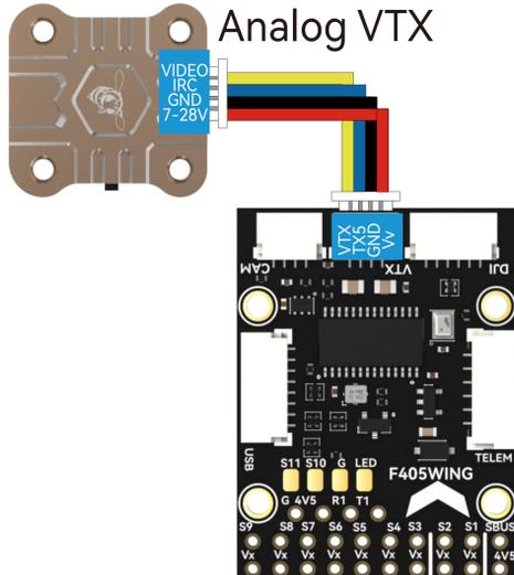
Note: Please adjust the VTX BEC power supply to 5V when using the TX800.
