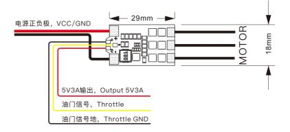
Voltage input/电压输入范围: 2~4S Lipo Continuous current/持续输出电流: 30A Max Current/最大电流: 35A Output/输出: Built in 5V 3A BEC/内置5V 3A BEC
