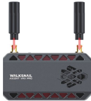
Installing the antennas on the RP-SMA ports
