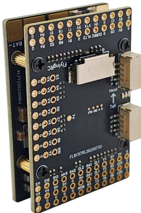
Assembly of the flight controller and the power board
