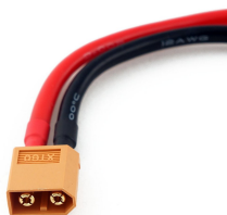
XT60 connector for connecting the battery
