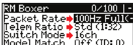
Obr. 1 – Packet Rate, Telem Ratio a Switch Mode v LUA skriptu ExpressLRS
