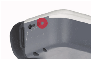
Bind button on the VTX (left) and on the goggles (right)
