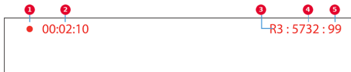
① recording ② recorded time ③ frequency position ④ frequency ⑤ RSSI
