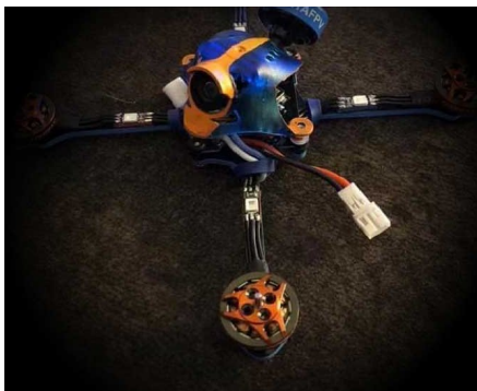
GTS V2 1202.5 series motors on a small FPV quadcopter (illustrative photo by the manufacturer).
